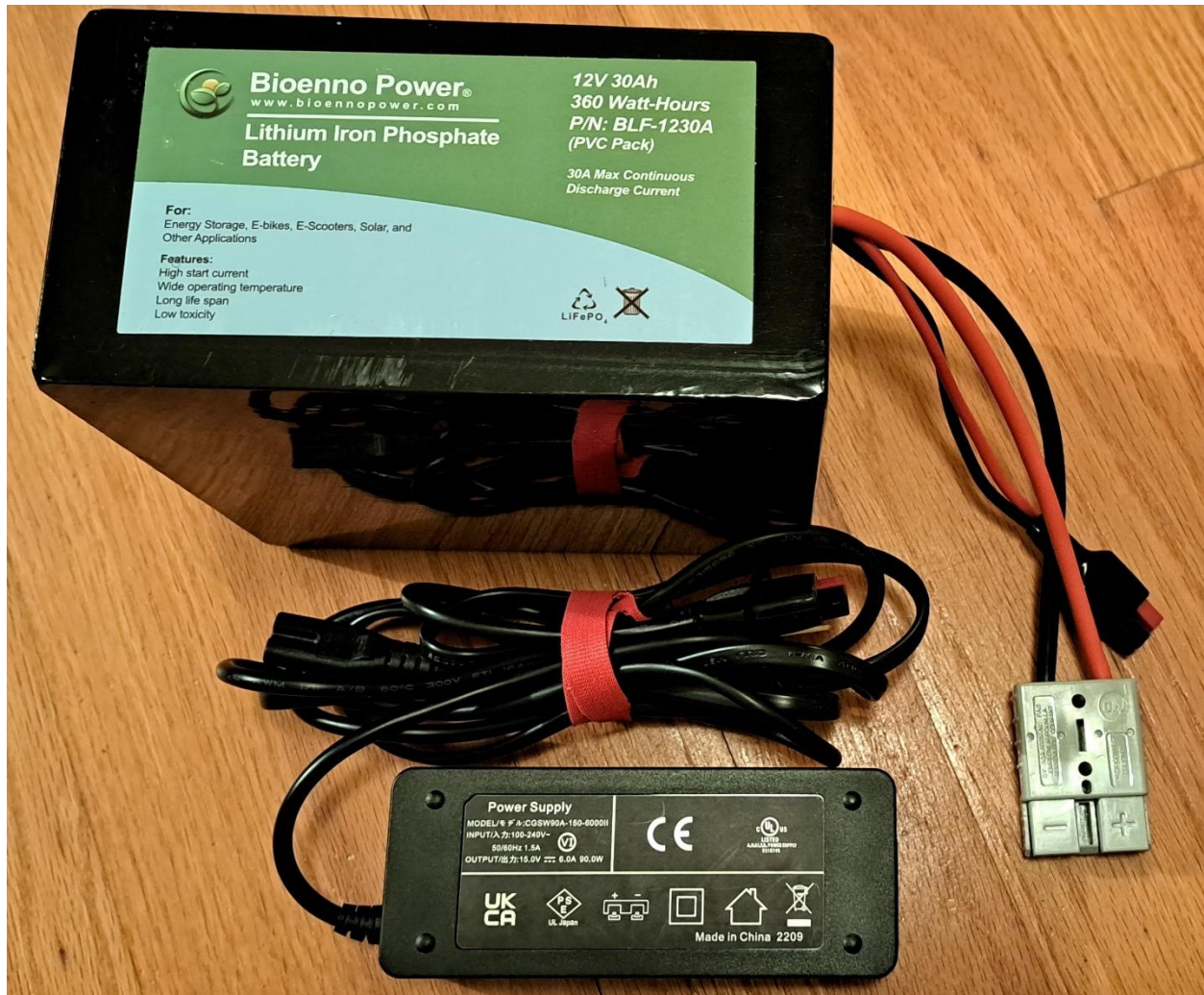
30Ah LiFePO 4 battery with charger (fits into battery box)
