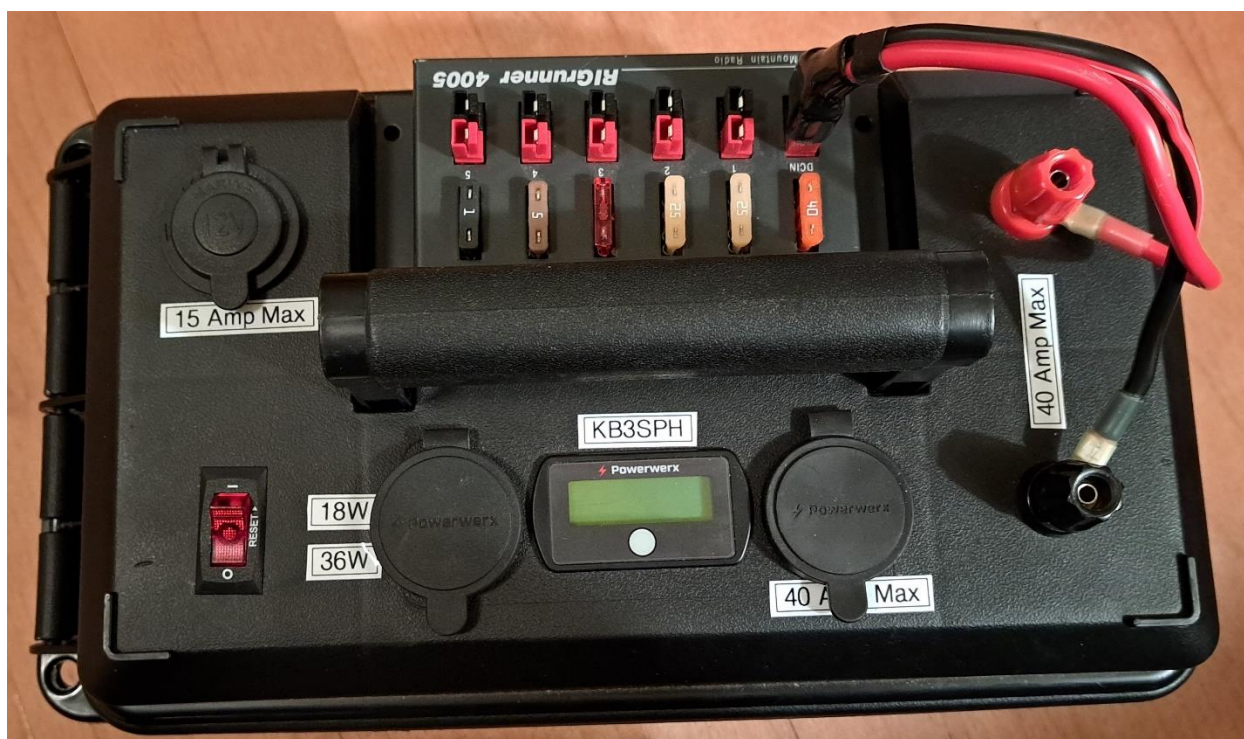
RIGrunner deployed. Powered via binding posts. Secured via Velcro under handle.
