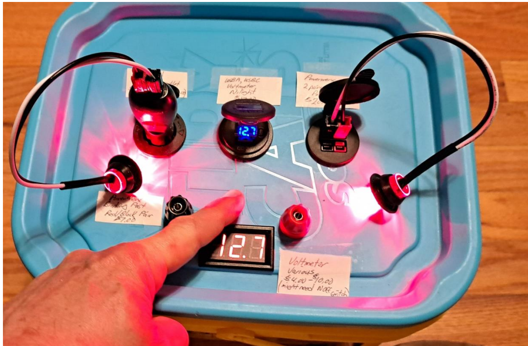
Cat litter battery box in operation! Finger pushing momentary switch to light the square voltmeter.
