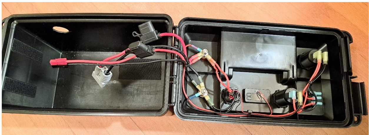
Empty battery box showing wiring harness. Extra hole in the side is for external solar panel and external power supply access to the PWRgate.
