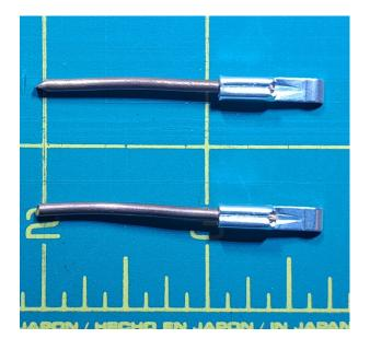
Insert Wires and Contacts into the pair of PowerPole housings
