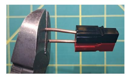
Clip both Inline Connectors onto the wires from the housings and ensure both fit flush.
