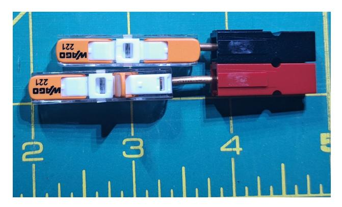
The wires in the kit are purposely cut long to allow variations in construction. The goal is to trim the wire so that there is no gap between the installed inline connector and the PowerPole housing. This will enable the strongest connection within the completed adapter. Notice the width of the gap and prepare to trim that amount of wire off of the end of each wire.
